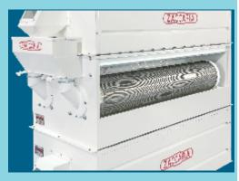
Obs: - Production capacity in kg/h is based in tests made from Brazilian long rice type; - The rice moisture recommended to obtain the maximum yield is between 12% to 13% (B.U.). - Equipment originally supplied with motor Indústrias Machina Zaccaria S/A reserves the right to change the information herein stated, including color and other details, without previous notice.
